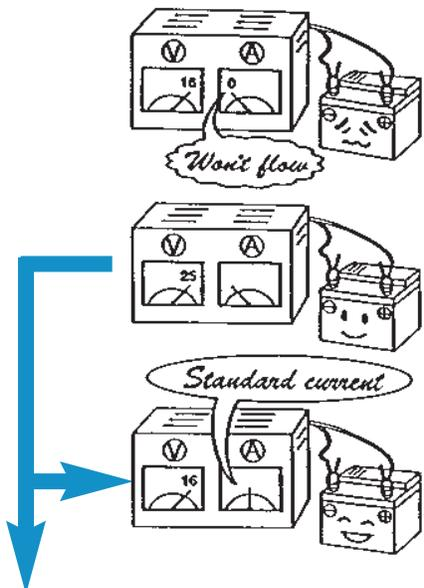
**Adjust voltage so that current will be at standard amps after 5 minutes.**
