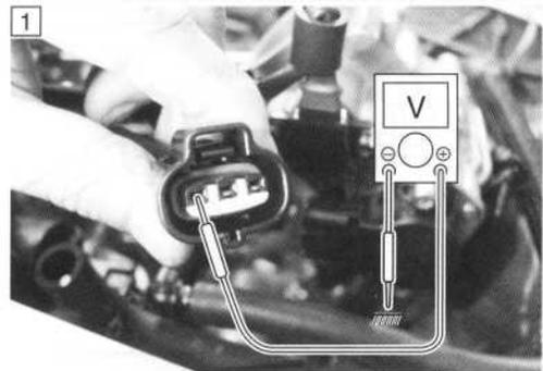
**DATA** TP sensor input voltage: 4.5 – 5.5 V
