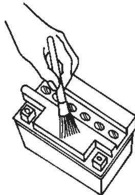
so cleaning materials don't get into cells and neutralize the acid.
