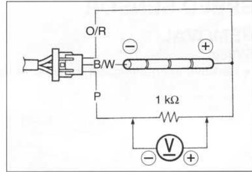
Lift and turn the front wheel and check that voltage varies between 0 – 6 V.
