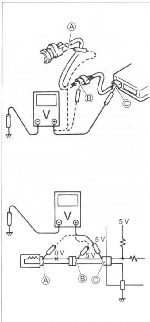
**SHORT CIRCUIT CHECK (WIRE HARNESS TO GROUND)**
