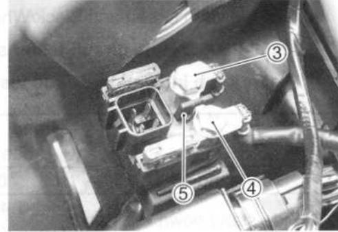
Apply 12 V to (A) and (B) terminals and check for continuity between the positive and negative terminals using the multi circuit tester. If the starter relay clicks and continuity is found, the relay is ok.
