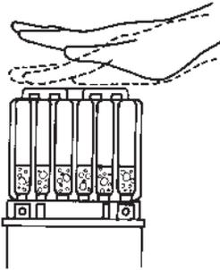
**4. Check the electrolyte flow. Keep the container in place for 20 minutes or longer until it empties completely.** If no air bubbles are coming up from the filler ports, or if container cells haven't emptied completely, tap the container a few times. Don't remove the container from the battery until it's empty. The battery requires all the electrolyte from the container for proper operation. Make sure the electrolyte container empties completely.
