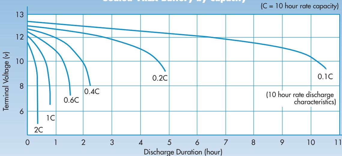
Starting the engine is a big part of the battery's job, but not all. Electrical accessories and safety systems – lights and horn – need a stable supply of electricity. Now you're concerned with the battery's "low rate discharge characteristics." This steady, low rate discharge is
