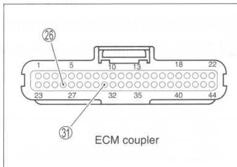
**“C32” or “C33” FUEL INJECTOR CIRCUIT MALFUNCTION**
