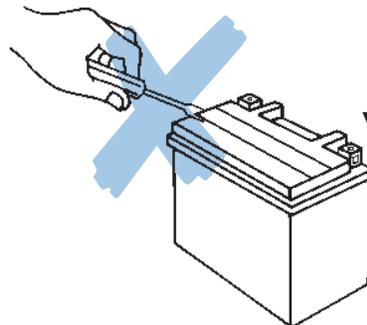
**Remember: unlike a conventional battery, the sealed VRLA battery won't be topped off during its life. Never pry off sealing caps: it's dangerous and damaging.**
