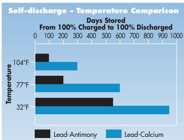
of 130°F are battery-killing. Been in a closed-up garage or storage building on a hot summer day recently? In many parts of the country, it's no trick for inside temperatures to reach that.
