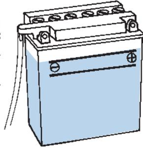
**5. Check the vent tube.** Make sure it's not kinked, pinched or otherwise obstructed. On a motorcycle, it should exit away from the drive chain and from below the swing arm. Small cuts in the tube near the battery vent are OK; they're an "emergency escape" for gas in case the tube becomes obstructed.
