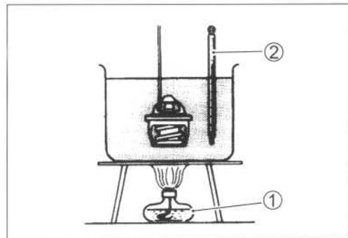
**DATA** Thermostat valve opening temperature
