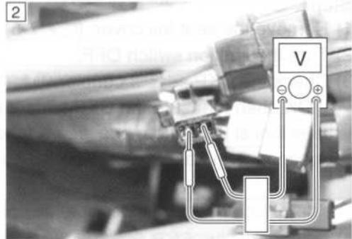
3) Repeat the above test procedure a few times and measure the highest peak voltage.
