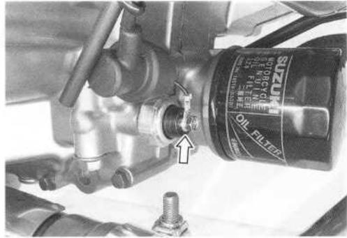
Check the oil pressure indicator lights, when grounding the lead wire.
