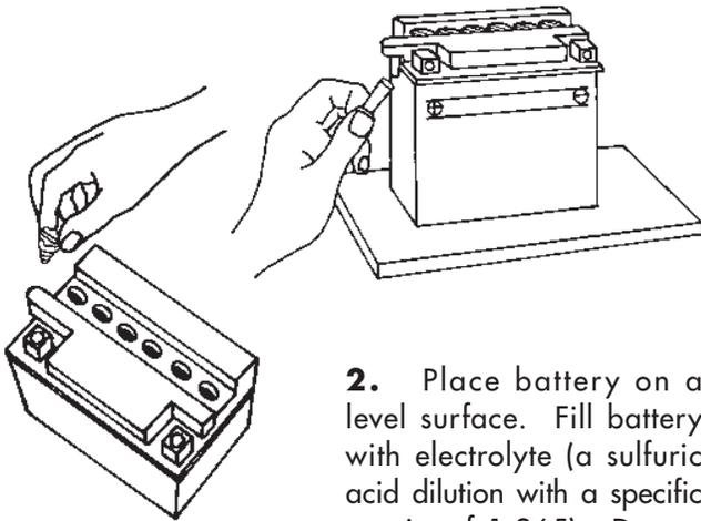
**2.** Place battery on a level surface. Fill battery with electrolyte (a sulfuric acid dilution with a specific gravity of 1.265). Do not use water or any other liquid to activate.
