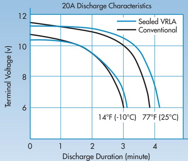
**Discharge Characteristics of a Sealed VRLA Battery by Capacity**
