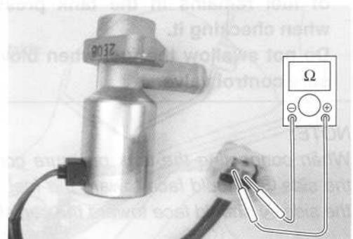
If the resistance is not within the standard range, replace the PAIR control solenoid valve with a new one.
