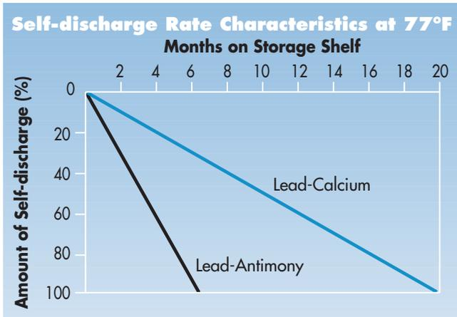
**Self-Discharge:** Self-discharge goes on all the time. It's a battery fact of life that they get weaker from "just sitting." How rapidly batteries self-discharge depends, first of all, on battery type. Lead-calcium batteries, such as YUASA's CX, YT, YI, discharge more slowly than conventional batteries. At room temperature lead-calcium discharges at 1/300 volt per day. Conventional lead-antimony batteries discharge at 1/100 volt per day.
