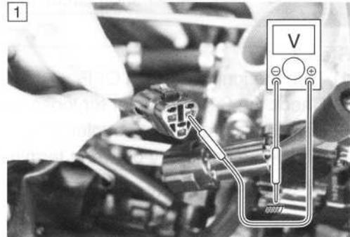
**DATA** STP sensor input voltage: 4.5 – 5.5 V
