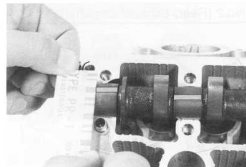
If the camshaft journal oil clearance measured exceeds the limit, measure the inside diameter of the camshaft journal holder and outside diameter of the camshaft journal. Replace the camshaft or the cylinder head depending upon which one exceeds the specification.
