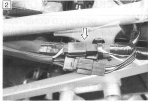
2) Crank the engine a few seconds with the starter motor, and measure the CKP sensor peak voltage at the coupler.
